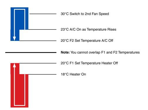
Example: Set Temperature F1 20°C, the controller will switch on the Heating if it is 18 degrees or less, and switch off the heater when vehicle temperature reaches 20°C.
