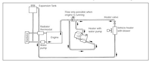
4. Instead of the thermostat in Example 1, an electrically operated changeover valve can be used for optional switching to small circuit (cab heating only) or large circuit (cab heating plus engine preheating).
