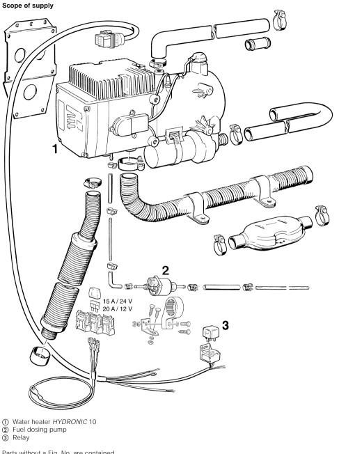
Parts without a Fig. No. are contained in the universal installation kit.
