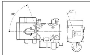
The water heater should be installed in the normal position shown in the diagram. The maximum permitted variation on this position is also shown. If any other mounting position is required, consult the manufacturer.
